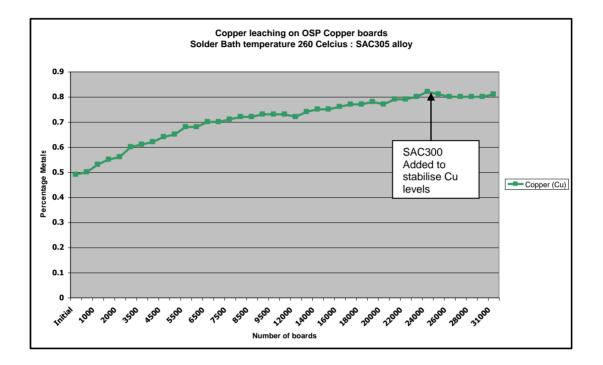
This shows an average leaching rate of **0.01% Cu per 1000 boards**. Each process is unique this is an indication only of the leaching rate (based on actual data).
